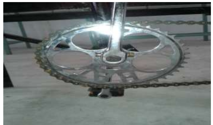
Fig 2: Driving wheel (diameter 18 cm)
