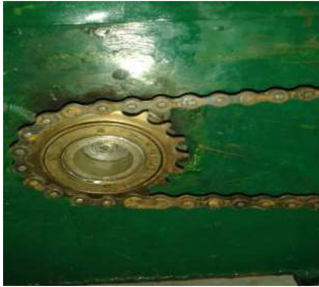
Fig: 4 Driven wheel (diameter 8cm)
